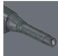
**Power trim & tilt switch and throttle grip friction adjuster**
